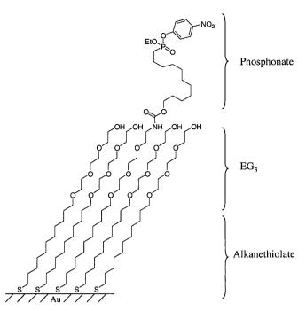
**Fig. 3.** Structure of a monolayer designed to covalently immobilize cutinase. The phosphonate capture ligand is present at a density of  $\approx 1\%$  of total alkanethiolate. After cutinase binds to the phosphonate capture ligand, an active-site serine residue displaces *p*-nitrophenol, resulting in irreversible covalent immobilization of the protein. The tri(ethylene glycol) groups prevent nonspecific protein adsorption to the monolayer.
