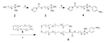
**Fig. 2.** Synthetic scheme for the phosphonate disulfide (**6**) used to prepare self-assembled monolayers. (a) CDI, CH<sub>2</sub>Cl<sub>2</sub>; (b) oxalyl chloride, CH<sub>2</sub>Cl<sub>2</sub>; 4-nitrophenol, Et<sub>3</sub>N, CH<sub>2</sub>Cl<sub>2</sub>; (c) **5**, Et<sub>3</sub>N, DMF.
